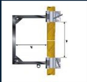
Alignment Clamp to prevent mechanical damage during separation of inner tubes
